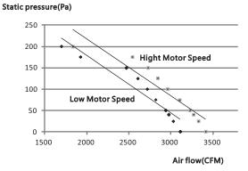
•Curve diagram of static pressure, air flow volumn
