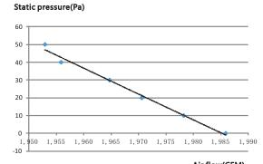
Air flow(CFM) •Curve diagram of static pressure, air flow volumn
