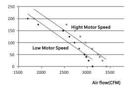
•Curve diagram of static pressure, air flow volumn
